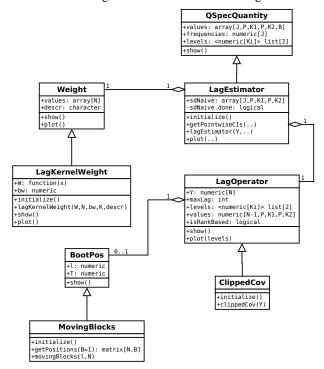
In the third class diagram the classes implementing model quantities are displayed. A relation to the "empirical classes" is given via the fact that the quantile spectral densities are computed by simulation of quantile periodograms and a common abstract superclass QSpecQuantity which is 6 quantspec-package
